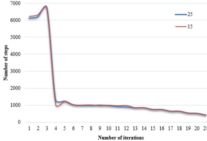
Fig. 3. Impact of sample data length on the convergence speed of the algorithm
