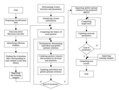
Fig. 4. Flow of improved BPNN under Bayesian classifier
