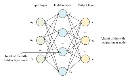
Fig. 3. Structure of the proposed BPNN
