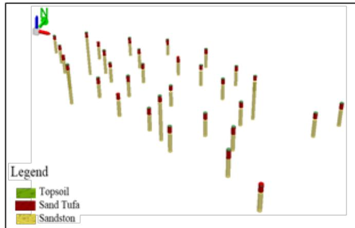
Fig. 7. Drilling data of study area
