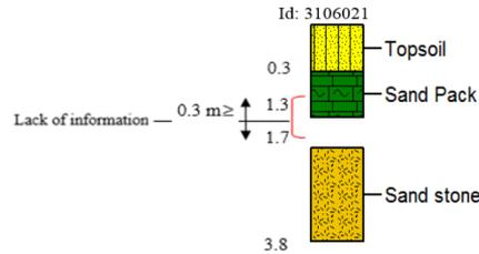
**Fig. 3.** Lack of information with a tolerance of 0.3 m or more
