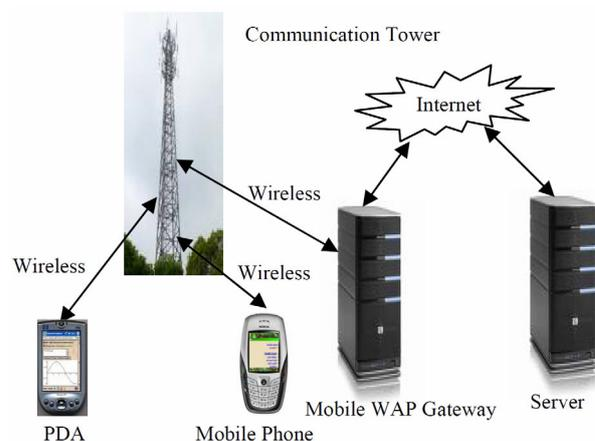
Figure 2. Internet-based mobile technology architecture.
