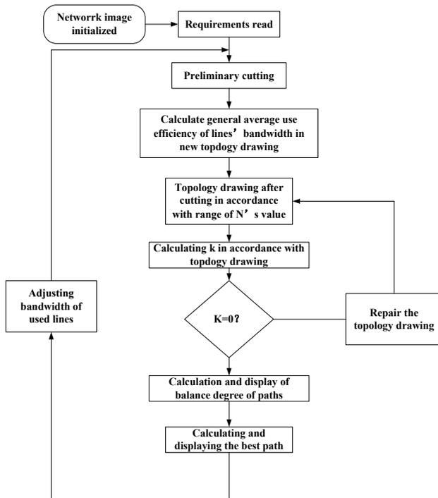
Figure 4. Dijkstra algorithm flowchart
