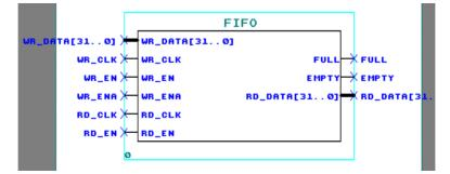
Fig. 11. FIFO module circuit design
