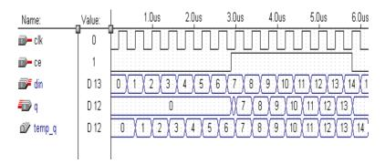
Fig. 8. Simulation waveform of Lock
