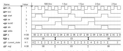
Fig. 4. Simulation waveform Control Module Design for ADC0809 Chip
