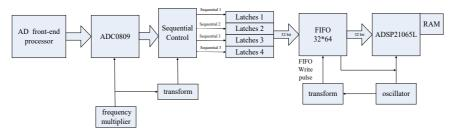
Fig. 1. Block diagram of data acquisition
