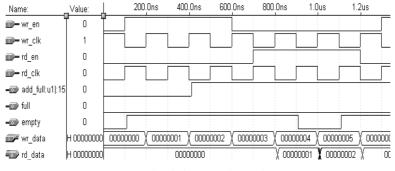
Fig. 12. Simulation waveform of FIFO
