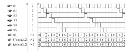
Fig. 10.Simulation waveform of clock conversion module
