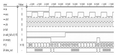
Fig. 3. The simulation waveform of this overall system program
