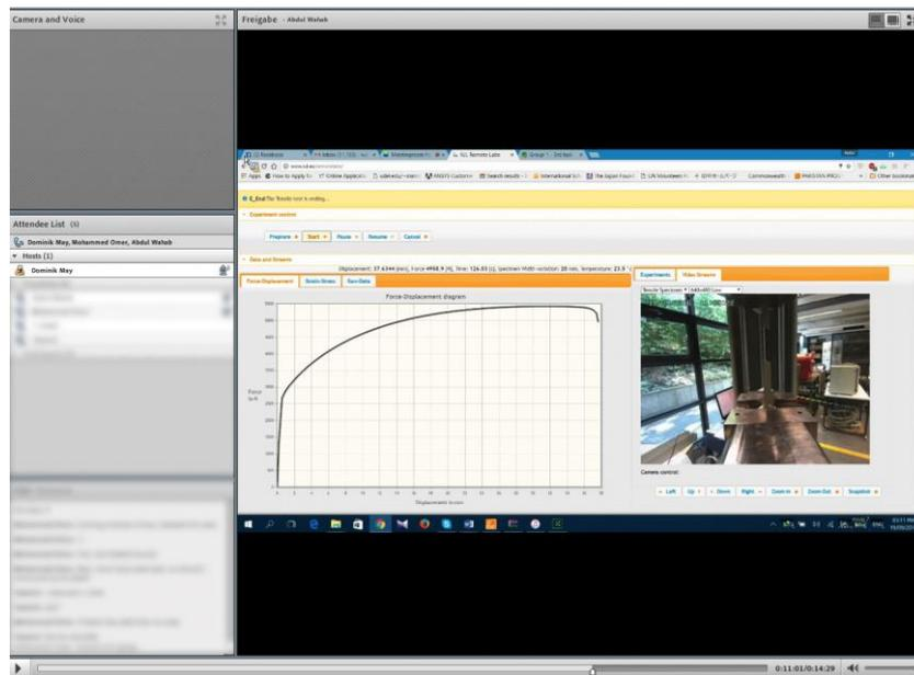
Fig. 4. Screenshot during the execution of a tensile test by students
