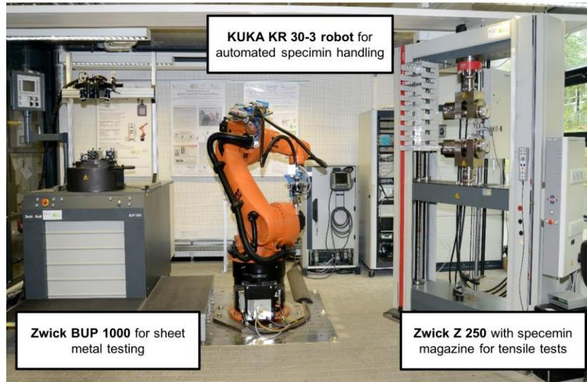
**Fig. 2.** Tele-operative testing cell at the IUL in the current expansion stage with two testing machines and one robot for automated test specimen handling
