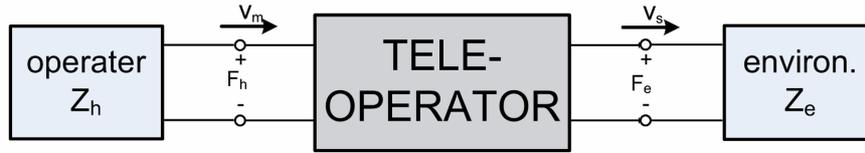
Figure 2. Network model of a bilateral teleoperation system
