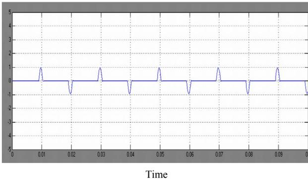
Fig 2a TCR Current Waveform with Alpha = 162 Degree
