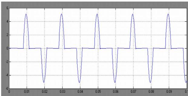
Fig 3a TCR Current Waveform with Alpha = 144 Degree
