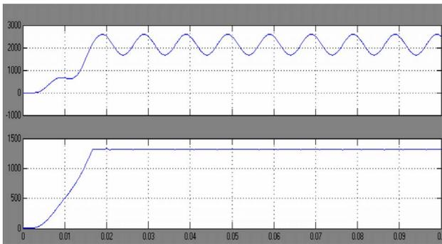
Fig 2b Real & Reactive Power with Alpha = 162 Degree
