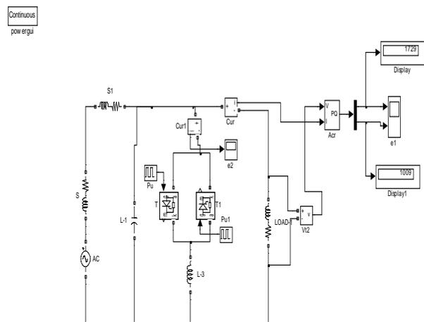
Fig 1b. Circuit model of FC- TCR
