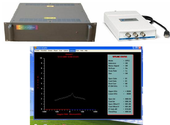
Figure 5. SpectraCyber digital receiver provided by RAS [21] (upper left) USB digitizer NI USB-5133 (upper right) and SpectraCyber software to analyze the hydrogen line spectrum.
