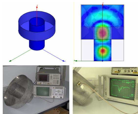
Figure 8. Development of the SRT horn feeding the parabolic reflector
