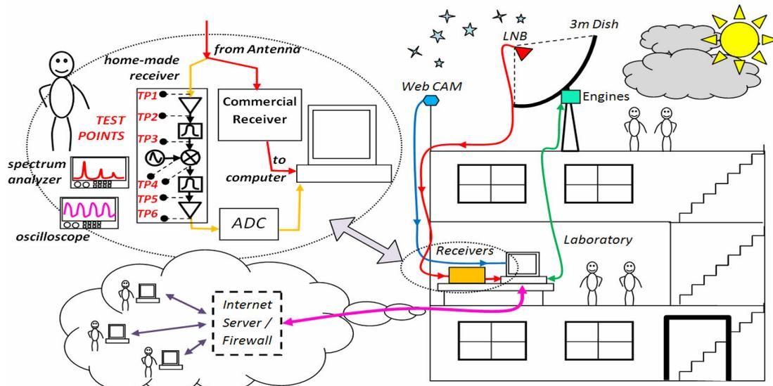
Figure 2. Scheme of the Radio Astronomy & Microwave and Antenna Engineering Laboratory
