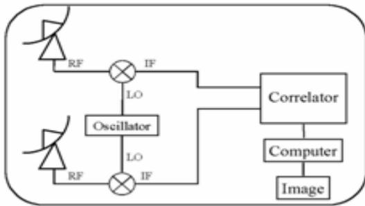
Figure 13. Scheme of a basic linked radio interferometer [11].
