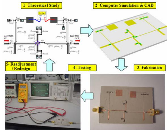
Figure 7. Development of a SRT microstrip low noise amplifier.
