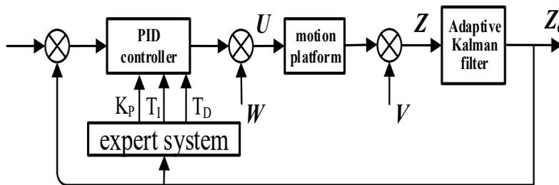
Fig. 6. Structural diagram of expert PID control algorithm based on adaptive Kalman filter
