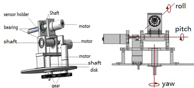
Fig. 3. The design of a 3-axis motion platform
