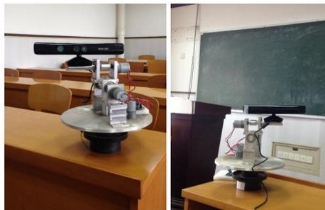
Fig. 4. A Kinect is installed upon the 3-axis motion platform
