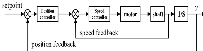
Fig. 5. Two-loop control structure with the speed loop nested inside the position loop
