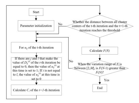
Fig. 4. Implementation flow of the improved fuzzy C-means algorithm
