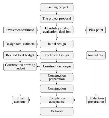
Fig. 10.Building construction procedure
