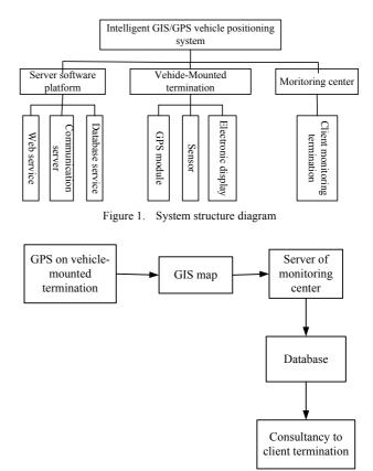
Figure 2. Data flow diagram
