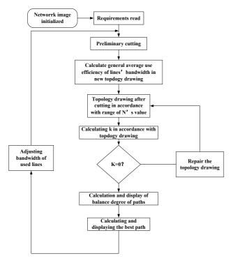
Figure 4. Dijkstra algorithm flowchart
