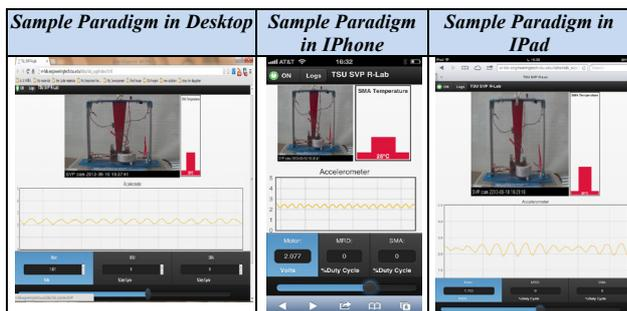
erometer output, which indicates the platform vibration, is shown in the middle of the Webpage. And the real-time video is displayed on the top of the Webpage. With our novel transmission solution, the real-time experiment video can be transferred to different terminal interfaces across the network firewall.
