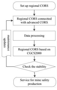
Figure 1. The technology process of CORS
