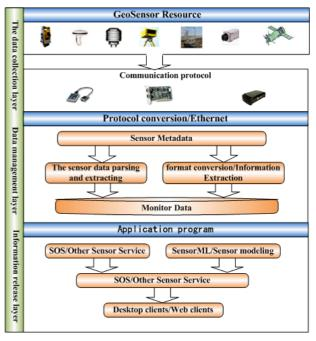
Figure 4. Multi sensor integration system framework for the ground disaster monitoring
