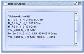
Figure. 6: Circuit Netlist
