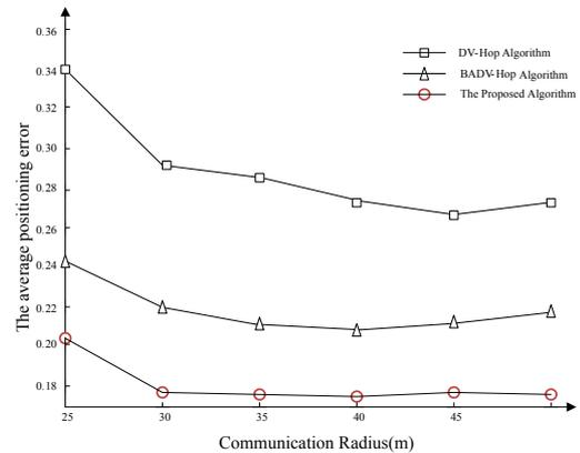
Figure 3. Communication Radius' Effect on the Positioning Accuracy
