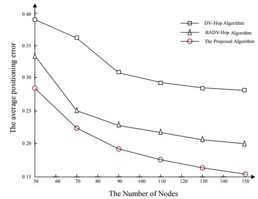
Figure 2. Number of Nodes' Effect on the Positioning Accuracy
