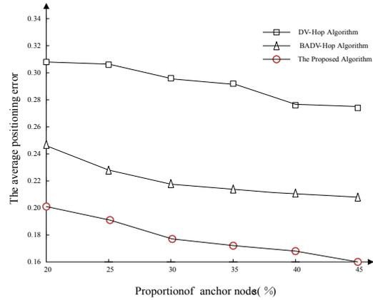
Figure 1. Anchor Node Ratio's Effect on the Positioning Accuracy
