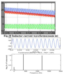
Fig.12 400Hz output spectrum at full rectifier load
