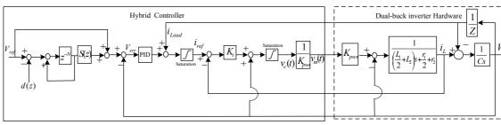
Fig.3 Block diagram of proposed hybrid control for AC voltage regulation
