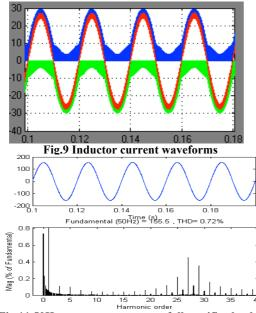
Fig.11 50Hz output spectrum at full rectifier load
