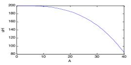
Fig.5 Nonlinear relation between the inductor current and inductance
