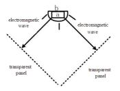
a is radar sensor, b is node of LED insect-trapping lamp
