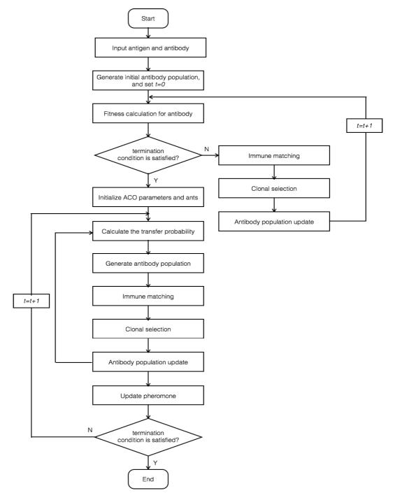
Figure 3. Workflow of proposed immunity based ACO algorithm
