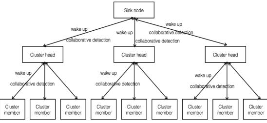
Figure 2. Overall structure of distributed intrusion detection in WSN
