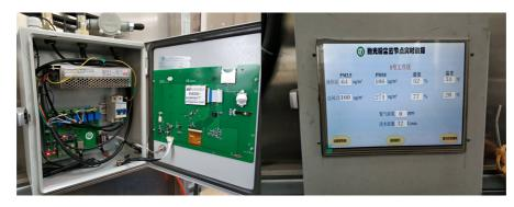
Fig. 13.Sink node with HMI
