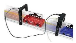
Fig. 6. Photo Gate Phasco Interface 750
