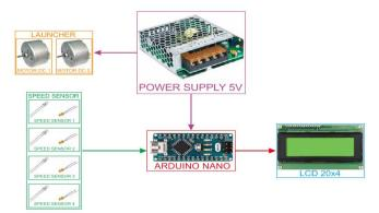
Fig. 1. Schematic Microcontroller Circuit
