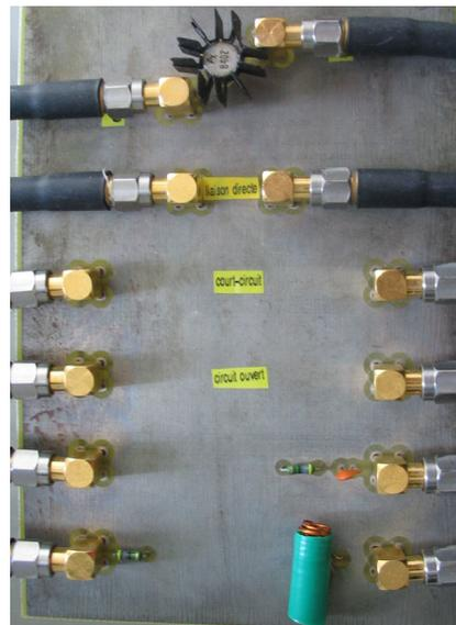
Figure 8. Picture of the "WebSwitch", a home-made device for switching from one component to be characterized to another.
