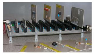
Figure 9. ISILab motherboard an experiments' cards
