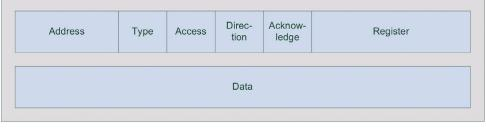
Figure 3. Format for packet based transmission
