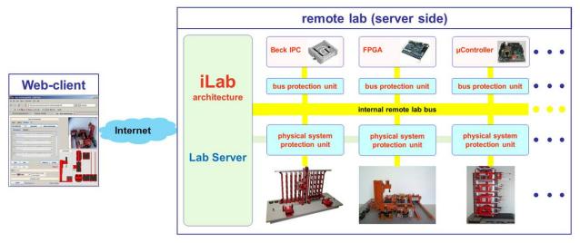
Figure 3. Grid architecture of the remote lab of the new REAL system (server side) with Web-client
