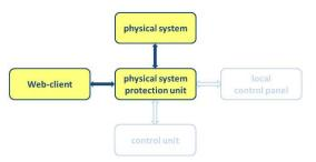
Figure 11. Remote control mode via a Web-client
