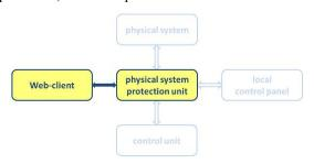
Figure 15. Virtual control mode to test the protection unit
