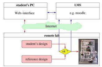
Figure 6. Observation of the student's design under LMS control
