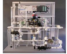
Figure 7. Simulation model and physical system of a water level control
