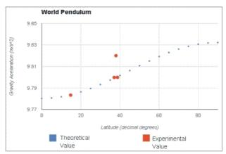
Figure 2. Estimated value of the 'g' acceleration with latitude variation. Showing the collected data points for each city.
