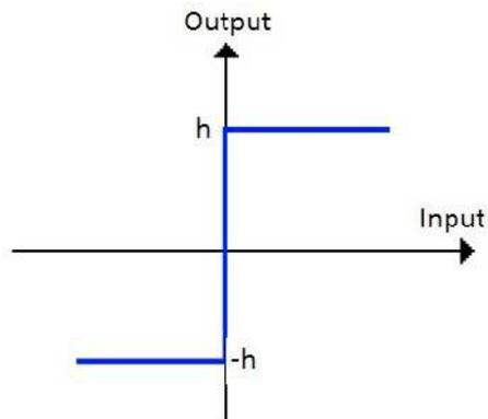
Figure 3. Relay output.
