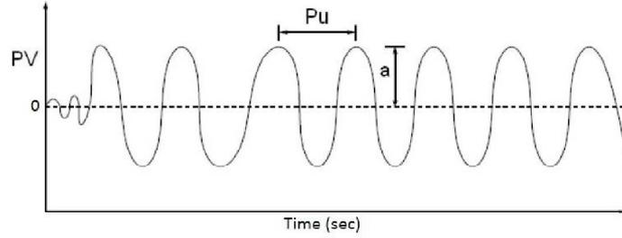
For a typical plant the oscillation obtained in the test occurring at the relay input is as shown in Figure 4. The critical frequency is taken as the measured frequency and the critical gain  $K_u$  is obtained by the formula,
