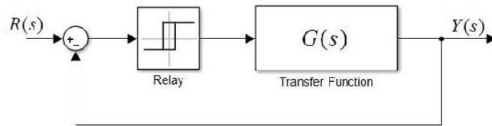
The relay method is based on determining the critical gain  $K_u$  and the critical frequency  $\omega_u$  (Yüce et al. 2016) as illustrated in the Matlab Simulink diagram of Fig. 1. The relay input-output characteristic is given in Fig. 2 and the relay output is shown in Fig. 3.
