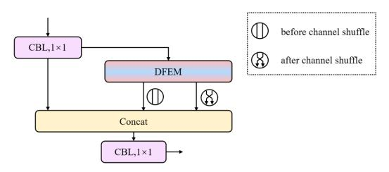
the ELAN module from the original YOLOv7-tiny backbone network with DFEM. They are connected by CBL blocks, enabling efficient extraction, separation, fusion, and activation of information of different frequencies in the input image. The output of the second DFEM (P1), the third DFEM (P2), and the end of SSPP (P3) of the backbone network are sequentially passed into the light-FPN, as shown in Figure 6.
