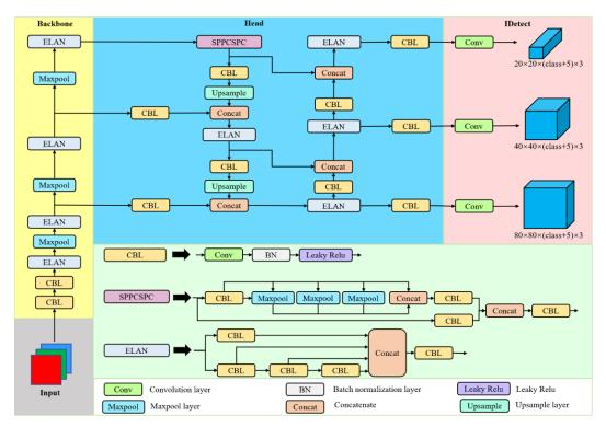
module replacement, model training, and model testing, a lightweight network model called YOLO-FLNet is proposed for applications with limited computing power. This model utilizes an efficient and lightweight backbone and a head structure capable of efficiently aggregating complex features (see Figure 2).
