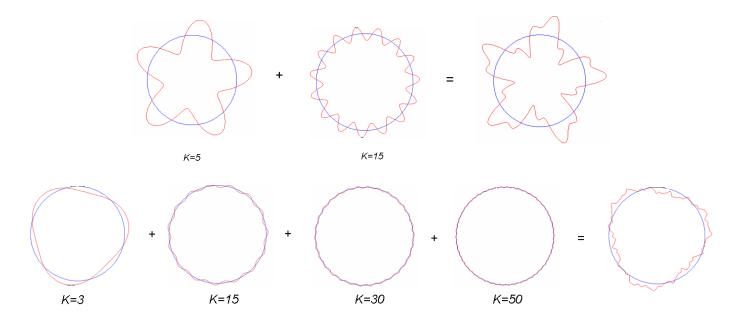
Fig. 1. Top: shape obtained as a perturbation of a circle at frequencies  $k = \{5, 15\}$ , with  $\hat{\delta r}(5) = 5$ , and  $\hat{\delta r}(15) = 2$ , where  $r_0 = 20$ . Bottom: shape obtained as a perturbation of a circle at frequencies  $k = \{3, 15, 30, 50\}$ , with  $\hat{\delta r}(3) = 1.5$ ,  $\hat{\delta r}(15) = 0.5$ ,  $\hat{\delta r}(30) = 0.3$ ,  $\hat{\delta r}(50) = 0.2$ , where  $r_0 = 20$ .
