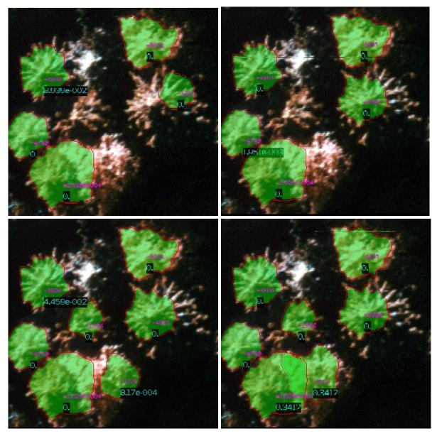
Fig. 4. Evolution of the configuration during the birth-and-death process. The objects are defined using the energy E, where g(k) is defined so as to discourage low frequency perturbations, and in particular the frequency k=2. Bottom right: final configuration obtained. The numbers on the crowns show the interaction term value  $H_2$  (black background) and the data term value  $H_1$ .
