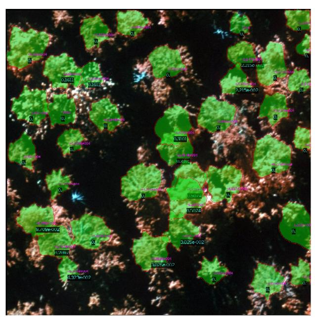
Fig. 5. Final configuration obtained (original CIR image of tree crowns,  $\odot$  CBA). The numbers on the crowns show the interaction term value  $H_2$  (black background) and the data term value  $H_1$ .
