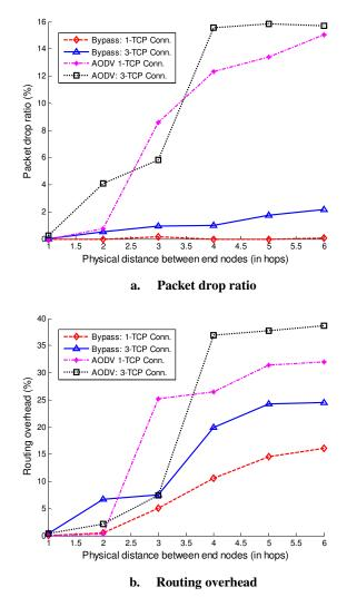
Figure 5: Packet drop ratio and routing overhead
