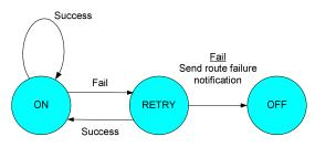
Figure 2: Channel state transition diagram
