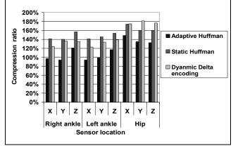
Figure 2. Compression ratios for entire 45 minute recording
