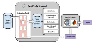
Figure 3. The EyesWeb XMI platform was adopted to perform tracking and analysis. The study of correlation between time series and statistical analysis was performed in Matlab and R.
