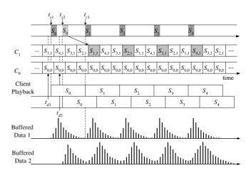
Figure 3: An illustration of segment downloading of HRAB when m = 4.
