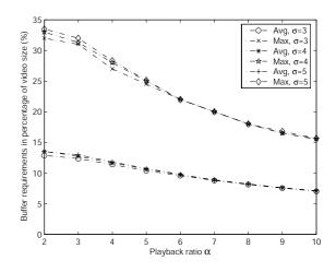
Figure 5: Comparison of required buffers of the HRAB normal case.
