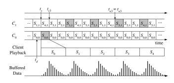
Figure 2: An illustration of segment downloading of RAB when m = 4.
