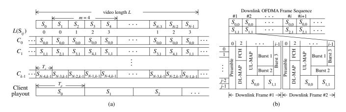
Figure 1: An illustration of the VoD system in WiMAX system; (a) the VoD program (b) the OFDMA downlink frame structure.
