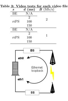
Figure 3: Testbed Schematic
