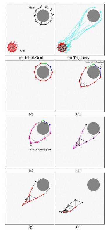
Fig. 7. Escaping from Type-III minimum. (a) Initial and goal formations. (b) Successful trajectories of all agents, with Backbone-based Leader-following strategies. (c)-(h) Snapshots of the system along the successful trajectories. (c) Backbone of initial formation, and all agents were in the backbone. (d) A local minimum detected. (e) Spanning tree was constructed. (f-g) Moving in leader-following mode. (h) Back to BBCC.
