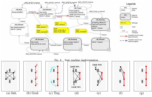
Fig. 5. Escaping from Type-I minimum. (a) Initial formation. (b) Goal formation. (c) Successful trajectories of agent #0 and #3 with Random Walk strategy. (d)-(g) Snapshots of the system along the successful trajectories. (d) Local minima detected by agent #0 and #3. (e) Agent #3 escaped the minimum, while agent #0 detected another minimum.
