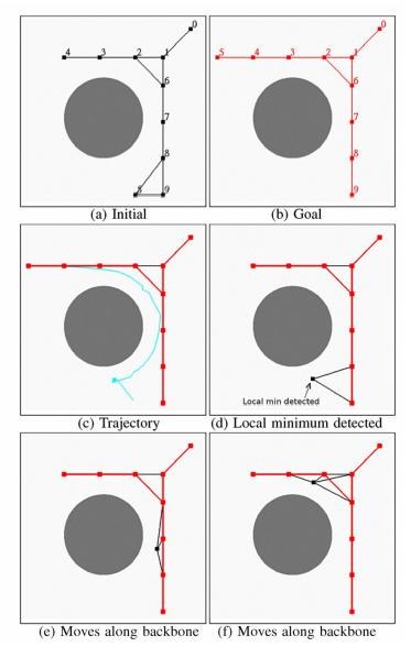
Fig. 6. Escaping from Type-II minimum. (a) Initial formation. (b) Goal formation. (c) A successful trajectory of the local minimum agent, with our Backbone-based Navigation strategy. (d) A local minimum detected. (e)-(f) Snapshots of the system along the successful trajectory.
