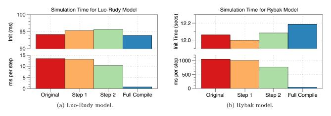
Figure 5: Comparison of execution time for different levels of compilation.
