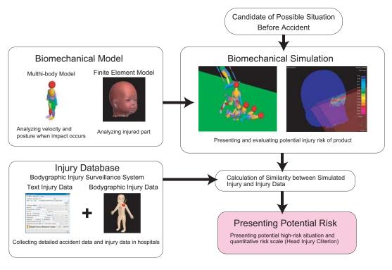
Figure 1: Configuration of the Proposed System
