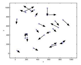
Figure 3: Randomly located links used in simulation. Arrows point from transmitters to receivers.
