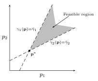
Figure 1: Illustration of  $p^*$  geometry for N = 2 case. The set of all feasible powers form a "cone" with the former point at its tip. Any other point in this cone satisfies  $p \ge p^*$  and thus requires greater power expenditure.
