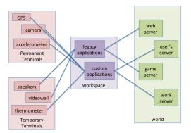
Figure 2: The system introduces a workspace between the client and servers.
