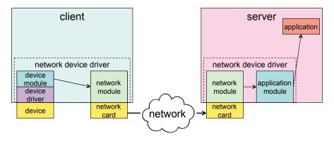
Figure 3: This data stream is sourced at the device and sinked at the application.
