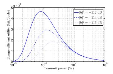
Fig. 1. Energy-efficient utility per user with respect to the allocated power for three different channel gains. Parameters are a = 1, and  $\sigma^2 = 5 \times 10^{-14}$  W.
