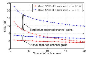
Fig. 6. Mean SNR of one mobile user with respect to the number of mobile users.
