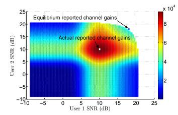
Fig. 4. Energy-efficient utility of the cell with respect to the SNR of users 1 and 2. The color bar represents the cell energy-efficient utility in bit/Joule. Parameters are a = 10,  $|h_1|^2 = |h_2|^2 = -112$  dB, P = 1 W, and  $\sigma^2 = 5 \times 10^{-14}$  W.
