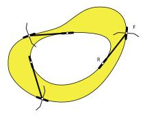
Figure 8: The area between front and rear tracks is  $\pi \ell^2$
