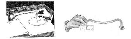
Figure 2: The Prytz Planimeter and its modification, due to Goodman
