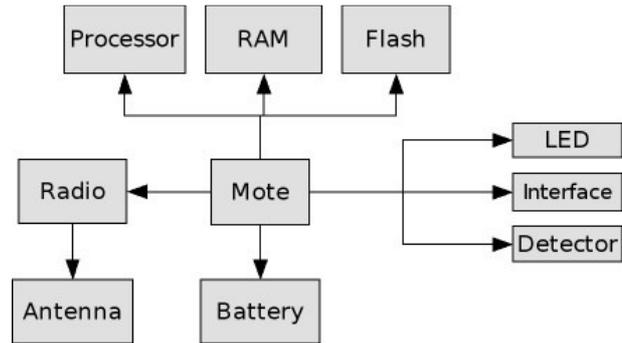
Figure 2. General architecture of a wireless sensor
