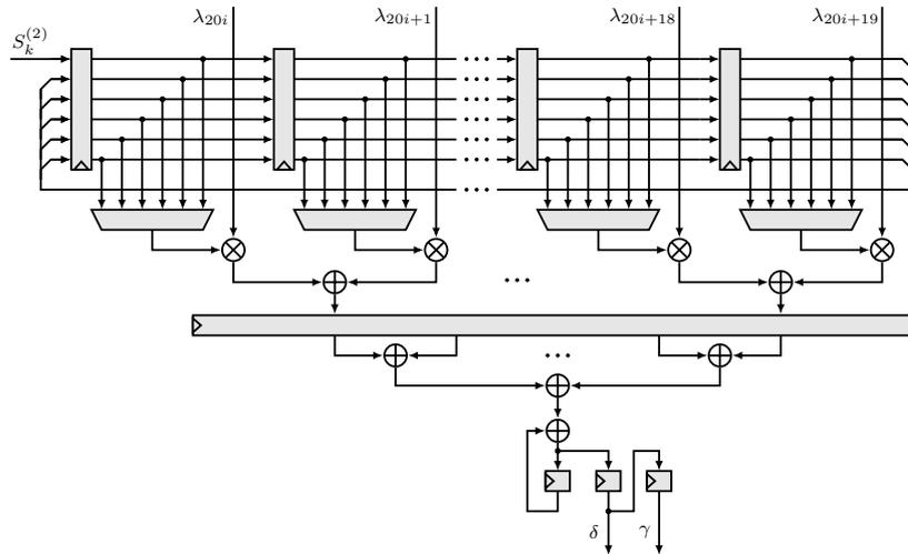
**Figure 3:** Block diagram of the iBM discrepancy computation module.
