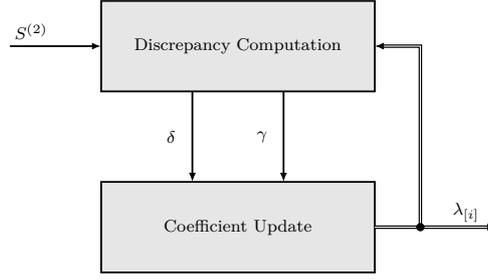
**Figure 2:** Block diagram of the pipelined iBM module, operating on blocks  $\lambda_{[i]}$  of the error-locator polynomial.
