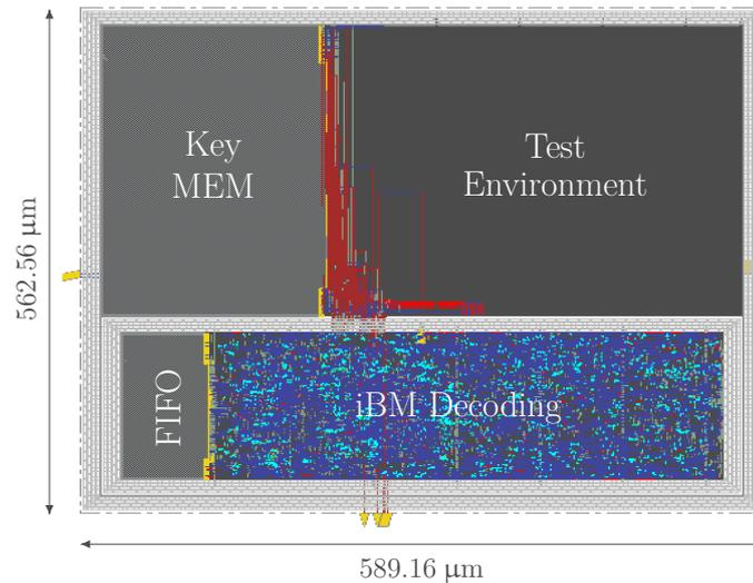
**Figure 6:** Layout of the iBM-based test chip with the test environment above the iBM decoding module containing the combined evaluation module’s FIFO.
