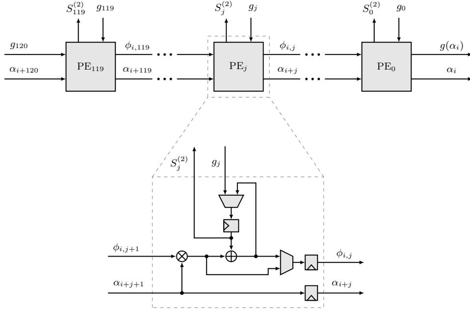
**Figure 5:** Block diagram of the combined systolic array (top) with detail view of the  $j$ th PE (bottom).
