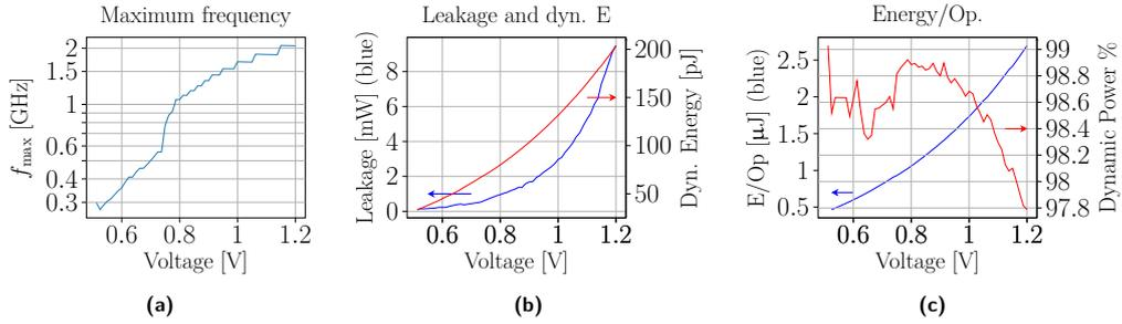
**Figure 8:** Measurement results of the iBM test chip: (a) Maximum clock frequency with verified correct decoding result. (b) Leakage power (blue) and dynamic energy (red) over  $V_{DD}$ . (c) Energy per decoding operation (blue) and percentage of dynamic energy (red) over  $V_{DD}$ .
