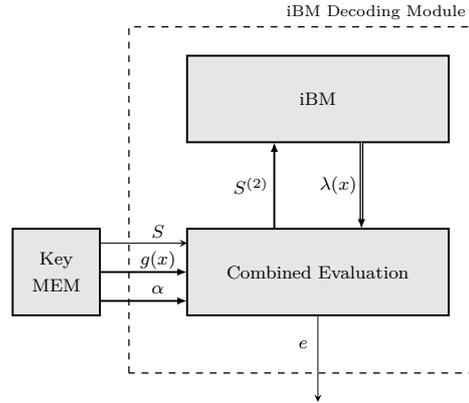
**Figure 1:** Overview of the proposed iBM-based Classic McEliece decoding architecture.
