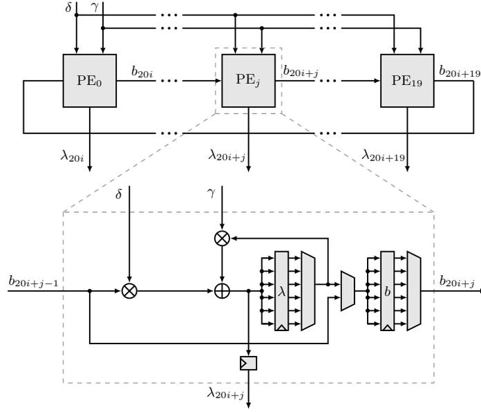
**Figure 4:** Block diagram of the iBM coefficient update module's systolic array (top) with detail view of a processing element (PE) at the bottom.
