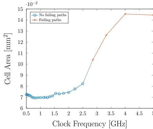
**Figure 7:** Clock frequency dependent cell area of the iBM decoding module with differentiation of design points with and without failing paths after synthesis.
