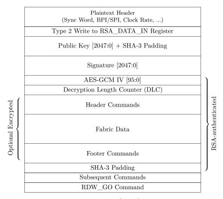
Figure 4: RSA Bitstream Structure based on [Pet21]. Gray-shaded words are written to the RSA\_DATA\_IN Register.
