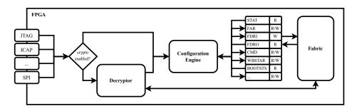
Figure 1: Our mental model of the configuration engine.
