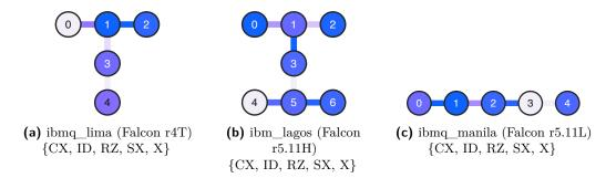
**Figure 11:** IBM Quantum computers used in the evaluation. Figure shows the device coupling maps. The color of nodes implies frequency (GHz, darker color means lower frequency) of the qubit. The connection color implies the gate time in nanoseconds for 2-qubit gates such as CX (darker color means shorter time).
