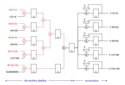
Figure 6: Architecture of the dot product pipeline.
