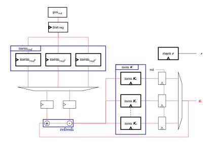
**Figure 5:** Architecture of the memory block.
