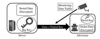
Figure 2: Leakage Resillient System with Whitebox Cipher and Network Monitoring
