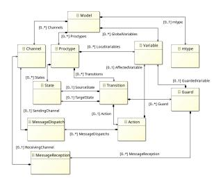
Figure 3: Class Diagram of the Promela Target Meta-Model
